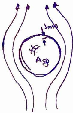
$$\begin{aligned} c &= 500 \text{ J/kgK} \\ \rho &= 700 \text{ kg/m}^3 \\ k &= 50 \text{ W/mK} \\ T(r_0, t) &= 1000 \text{ K} \\ Q &= 0,020 \text{ m} \\ T_i &= 300 \text{ K} \end{aligned}$$
